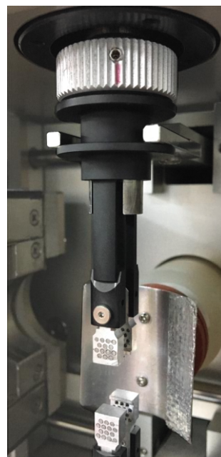
Fully Automatic chuck of VR-7130
