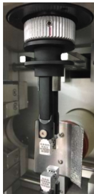
Fully Automatic chuck of VR-7130
